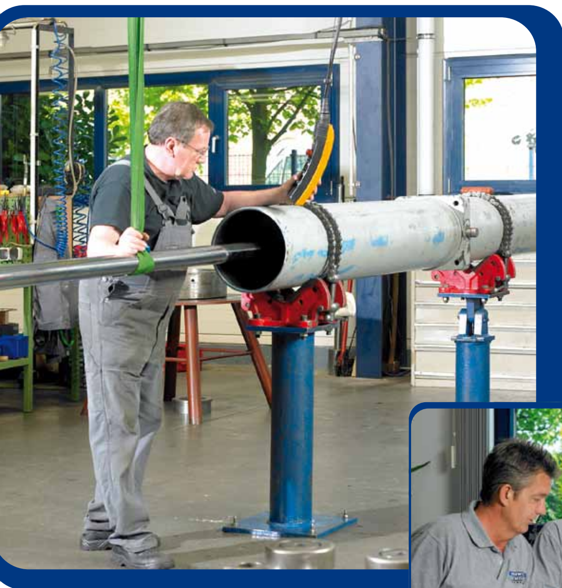
Disassembly of a dual-action cylinder on specially produced chain vices.
